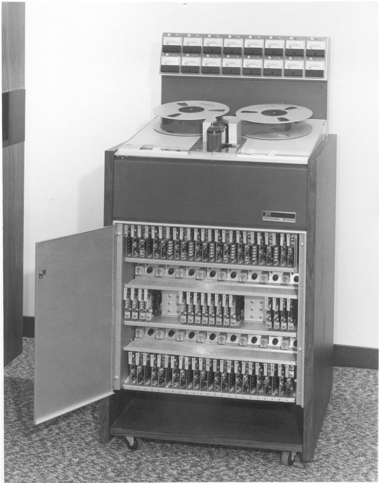
Model 56 Prototype Note single door, small casters, two erase capacitor mounting plates
