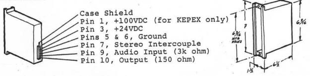
An external power supply is required, delivering 24VDC at 70mA for each GAIN BRAIN module. The LX-100 power supply by Allison Research is recommended, which provides the necessary power to drive up to eight modules (and includes a 100VDC terminal required for KEPEX 500 modules). The power transformer may be strapped for 105-125 or 210-250VAC, 50-60Hz operation. Instructions are provided with each LX-100.
