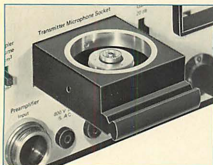
Fig. 4. Transmitter microphone socket with standardized ground shield
