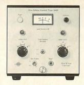
use). The positive and negative acceptable deviation limits may be set independently to 1, 3 or 6 dB, or switched off independently. The smoothing circuit which integrates the immediate history of the control signal has a frequency-dependent time constant, with a choice of two multipliers for use in installations with up to three control signal measuring positions multiplexed in the Control Signal Selector Type 5686.
