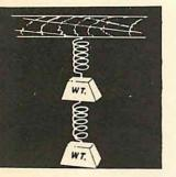
Even with an exceptionally quiet motor, it was found necessary to use a double mounting to absorb all detectible vibration. This mounting employs a twosection, low-pass mechanical filter. Standard components of proven reliability have been used for long and trouble-free life.
