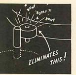
The elimination of rubber idlers thru the use of direct belt drive assures a permanent smooth drive system. Speed change is quickly made by placing the endless belt on the proper stepped pulley. Long periods of idleness will not affect the endless belt adversely. At 60 cycles line frequency, the absolute speed is held within 0.25%.
