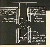
Reduction of metal-to-metal contact by the use of a nylon sleeve bearing gives smooth and quiet operation. The nylon requires negligible lubrication. The bottom thrust ball rides in a special hardened and polished seat. The extremely low friction, as a result of the above bearings, assures maximum benefit from the 25 pound turntable in stabilizing the turntable speed.
