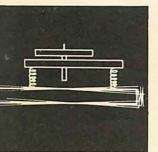
The entire turntable assembly is suspended on four coil springs equipped with felt dampers to absorb floor and cabinet vibration. This system minimizes the likelihood of feedback from the loud speaker, rumble from street traffic, oil burners, etc.
