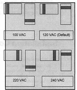
Fuse location and Input power voltage selection. The fuse is located directly behind the IEC Power input connector. There are two internal switches with which the input voltage range can be set to accommodate anything between 90 and 250 VAC. Please leave this adjustment to qualified personnel. When in doubt, call the factory!
