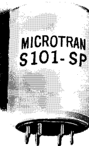
Fig. -SP PRINTED CIRCUIT MOUNTING Double Mu-metal shielded. 3/4"D x 1 1/8"H. 7-.040 pins. 3/8"H.
