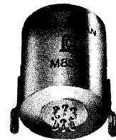
Fig. BB: HERMETICALLY SEALED to meet MIL-T-27. Triple mu metal case, high compression glass terminals, 6-32 x 3/8" mounting studs on 1/2" centers; 1" dia. cut out for terminals. Weight: 5 oz.
